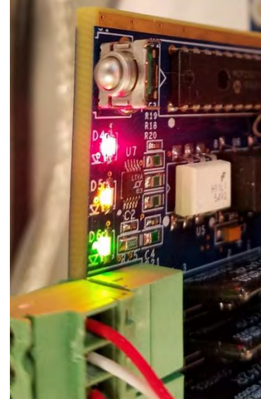
Figure 21 - Relay Module LEDS
